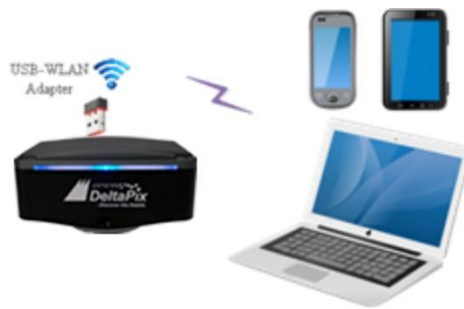
Figure 4-2 The PC or Mobile Device Connect to the Camera through WLAN
